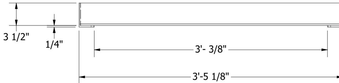
1. MATERIALS AND MANUFACTURING METHODS SHALL CONFORM TO ASTM C-913 AND ASTM A-36.
