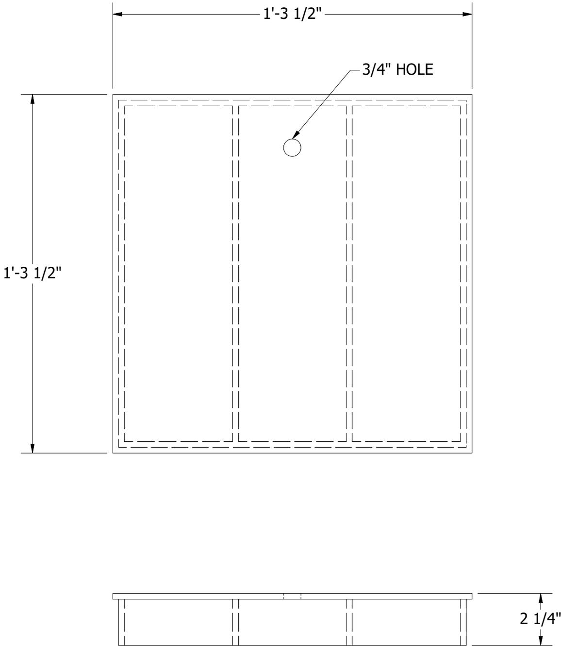
1. MATERIALS AND MANUFACTURING METHODS SHALL CONFORM TO ASTM C-913 AND ASTM A-36.
